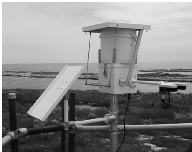
Closed cover sealing sample collection container
