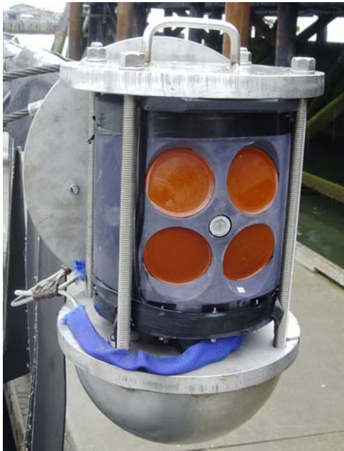
Figure 3c,d: At left in c) a close-up of ADCP head. At right in d) the pole-mounted Remus 1200 kHz ADCP (shown with pole retracted for transport). The first bin of good data is at 3.7 m nominal depth.
