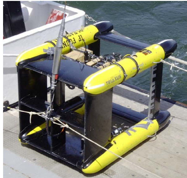
Figure 3a,b: At left in a), two views of the Triaxus towfish, showing the LOPC (A), LISST-100 (B) and the two OS-200 CTDs (C). The Remus-configuration 1200 kHz ADCP is mounted in the top right pontoon and looks upward; it is visible at right in b).
