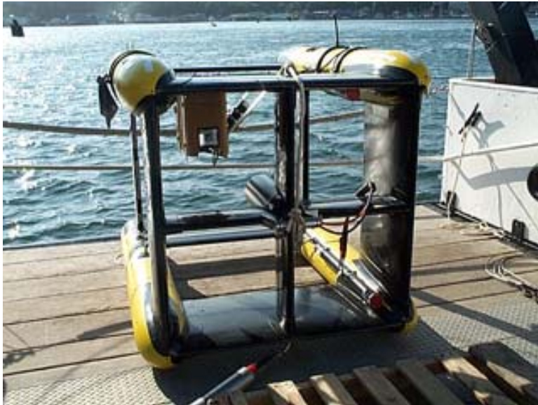
Figure 3a: The Triaxus towfish, showing the two OS-200 CTDs and LOPC; the Remus-configuration 1200 kHz ADCP is mounted in the top right pontoon and looks upward.
