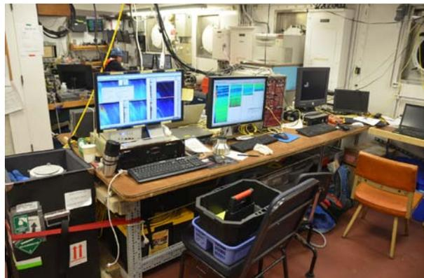
**Figure 9.3.1** - Acoustic control area. HTI deck unit (red) on right with control computer immediately to the left. Edgetech deck unit and control computer to far left. [Photo: P. Wiebe]
