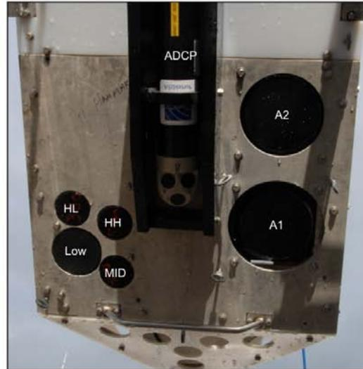
**Figure 9.4.1** – Edgetech channel assignments and other settings [Photos: P. Wiebe]
