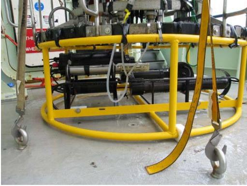
Fig. 9.2.3. Side view of the VPR in its cage under the CTD rosette. [Photo: N. Copley]
