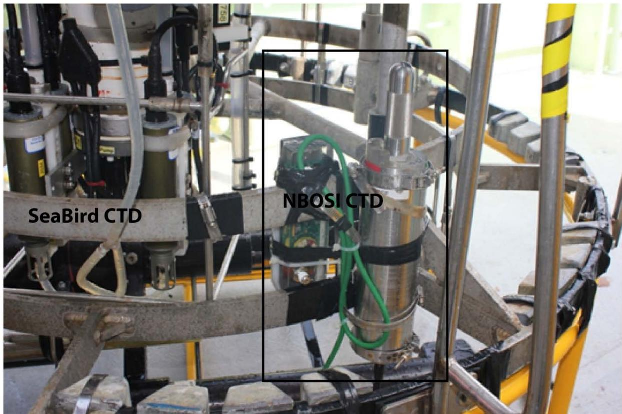
Fig. 13.1. NBOSI CTD mounted on rosette frame. [Photo: N. Copley]
