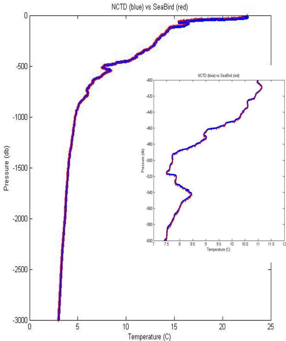
Fig. 13.2. Temperature trace for both the SeaBird and the NBOSI CTD's from cast 36, station 21.
