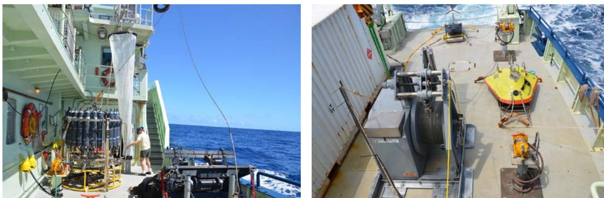
**Figure 6.1** – Main deck layout. Left: Working deck layout, with CTD aft of wet lab and MOCNESS propped up on its crutch next to the starboard rail. Right: Fantail layout, showing storage van (starboard side), Dynacon portable winch, HammarHead towed body (aftmost), and Greene Bomber towed body (port side). [Photos: P. Wiebe]
