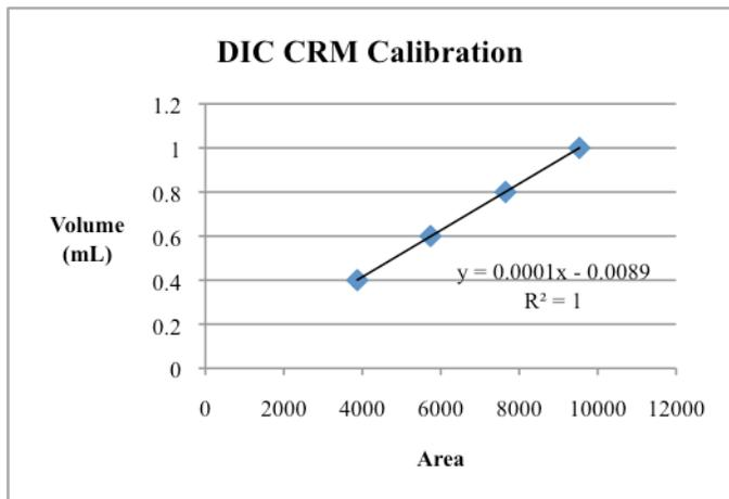
Fig. 8.2. Calibration curve of the DIC measurement.
