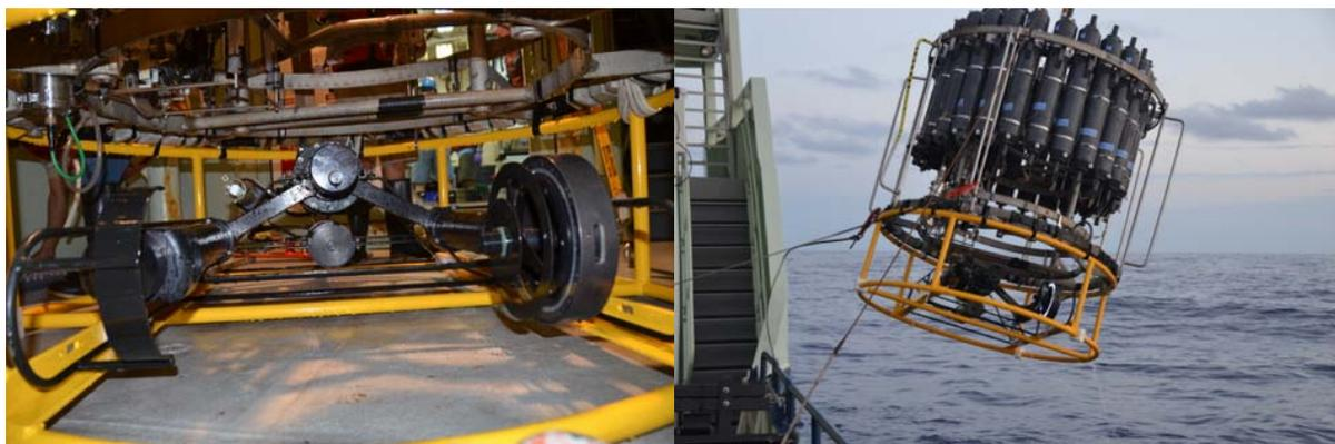
Fig. 9.2.1 The VPR installed beneath the CTD rosette. [Photo: P. Wiebe]
