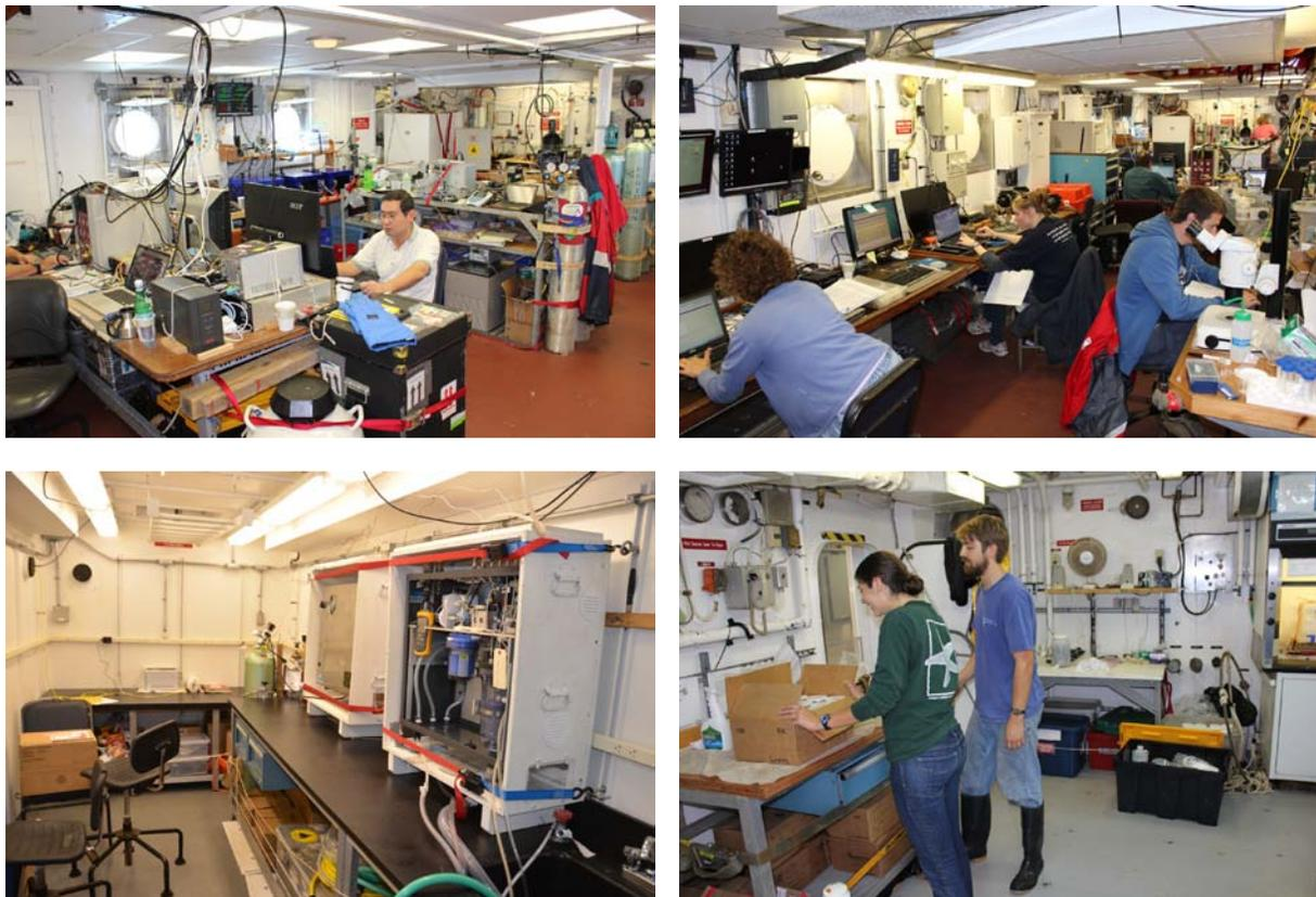
**Figure 6.2** – Lab layouts. Clockwise from top left: Forward portion of main lab with acoustic and chemistry areas; aft portion of main lab with microscopes (right) and VPR/MOCNESS computers (left); wet lab; science van with GO PCO<sub>2</sub> system. [Photos: G. Lawson, except P. Wiebe for van shot]
