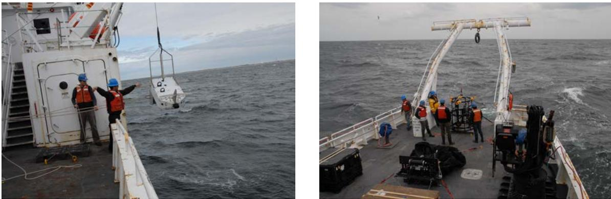
Figure 6.1. Main deck layout showing the deployment locations of the HammarHead (left) and MOCNESS/VPR-CTD (right). Photos: P. Wiebe.
