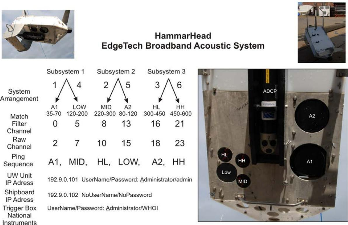
**Figure 8.2.1** – Edgetech channel assignments and other settings [Photos: P. Wiebe]
