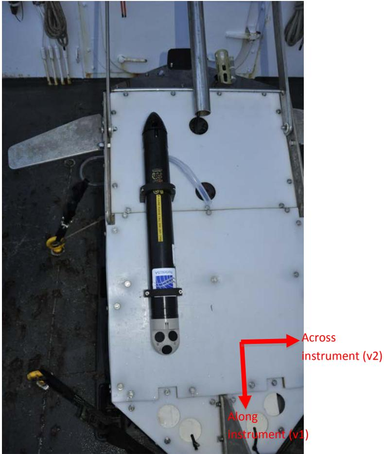
*Figure 7.4.* Nortek mounted upward-looking on the HammarHead. Arrows indicate instrument coordinate system. The z-coordinate (v3) is straight up (out of the page). The coordinate system is the same relative to the instrument for the downward-looking deployment. Photo: N. Woods.
