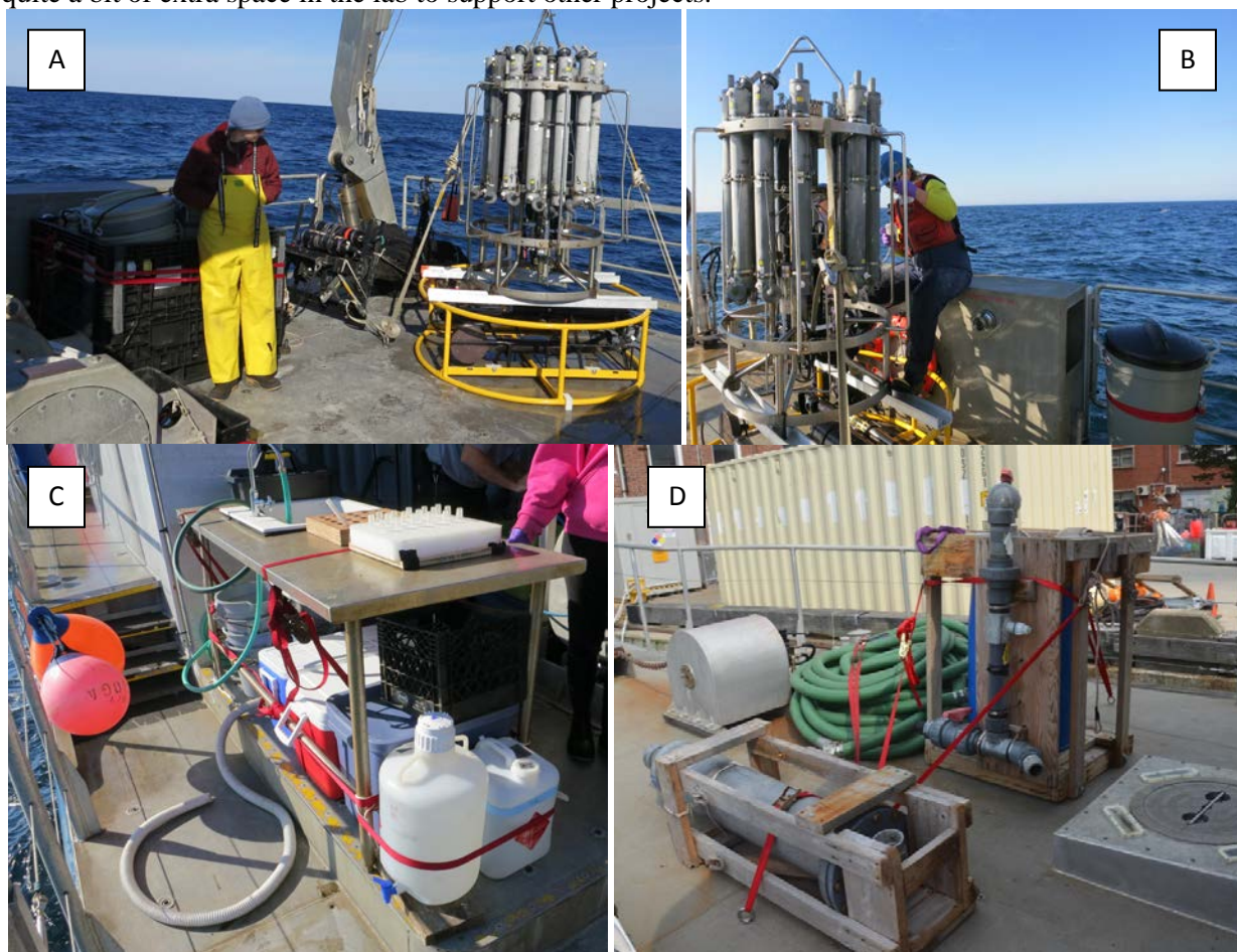
Figure 2 –A) Configuration of the back deck featuring the VPR on its modified housing below the CTD, the ¼ m MOCNESS on the starboard side, and the collapsible pallet containing the four trash bins. The Reeve net was strapped to the aft part of the collapsible pallet (not shown here). When the back deck was being used for other things the CTD was moved forward and to the port side. This is also where the extra trash cans were strapped down. C) The sink was set up on the port side of the back with the ethanol on the outside for ease of access. The in-use carboy was propped up on a piece of wood. D) Configuration of the starboard side of the forecastle with the gear associated with the large pump, excluding the generator Photos by: Peter Wiebe
