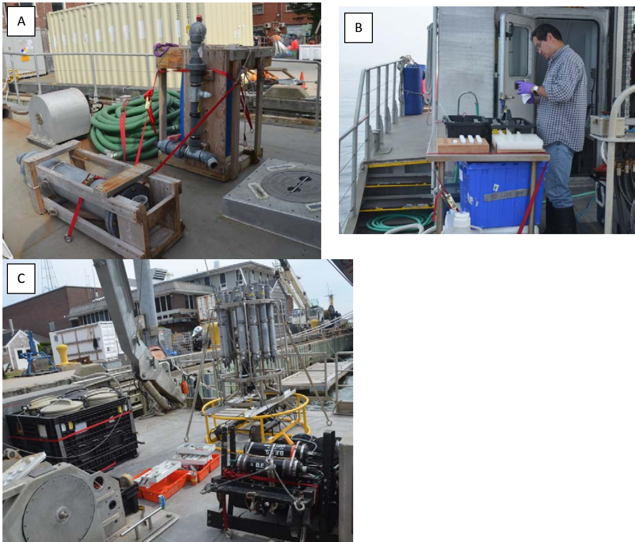
Figure 2 – A) Configuration of the starboard side of the forecastle with the gear associated with the large pump, excluding the generator. B) The sink was set up on the port side of the back C) Configuration of the back deck featuring the VPR on its modified housing below the CTD, the ¼ m MOCNESS on the port side, and the collapsible pallet containing the four trash bins. The Reeve net was strapped to the aft part of the collapsible pallet (not shown here) Photos by: Peter Wiebe
