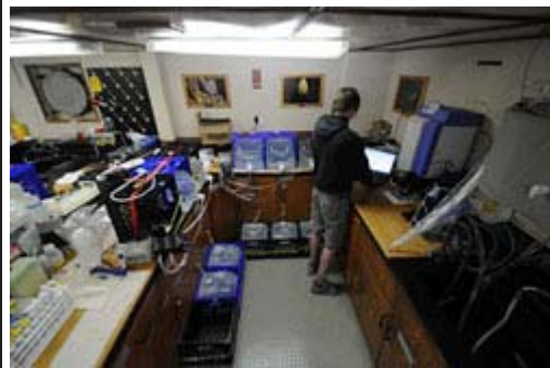
The lab space on R/V KOK has been configured to do many things and to remain safe in heavy weather. This corner is devoted to both processing water samples, which are lashed to the counter and floor, for cesium analysis and to Jarvis Caffrey's station radiation monitoring station. (Photo by Ken Kostel, Woods Hole Oceanographic Institution)
