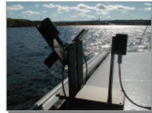
The MicroSAS can be mounted on ships of opportunity, small planes and helicopters.
